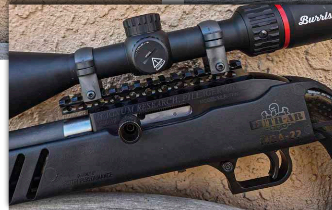
The bolt handle is oversized and easily operated with the support hand while keeping the rifle shouldered. The SwitchBolt also has a bolt hold-open button. The only gripe with this rifle is the magazine release can be a little challenging to operate, but with practice, smooth reloads can be conducted.
