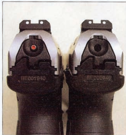
The visible/tactile cocking indicator protrudes from the rear of the pistol when the striker is cocked in single-action mode.
