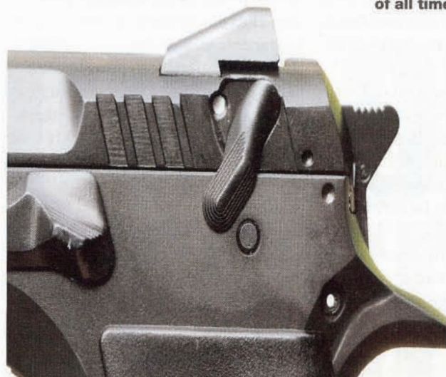
▲ The pistol's safety drops the hammer and also de-links the trigger from the firing system, so if it's in the down/Safe position, the gun will not fire.
