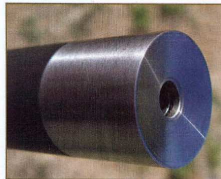
A stainless end cap (above) protects the muzzle and locks in the carbon fiber cover. The forged and machined receiver (below) sports an integral and racy-looking optic's rib.
