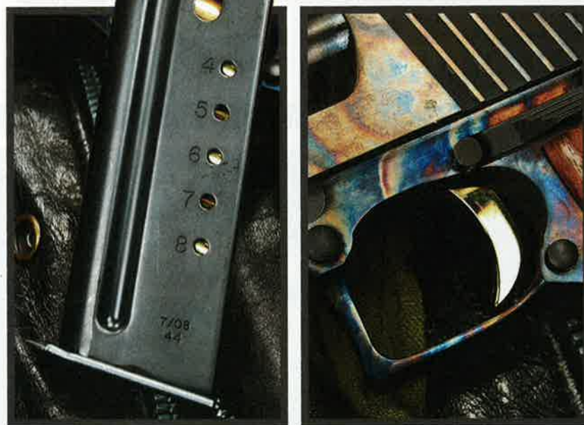
↑ The pistol comes with a steel, eight-round magazine. Also note the gold-plated trigger inside the large, squared triggerguard.
